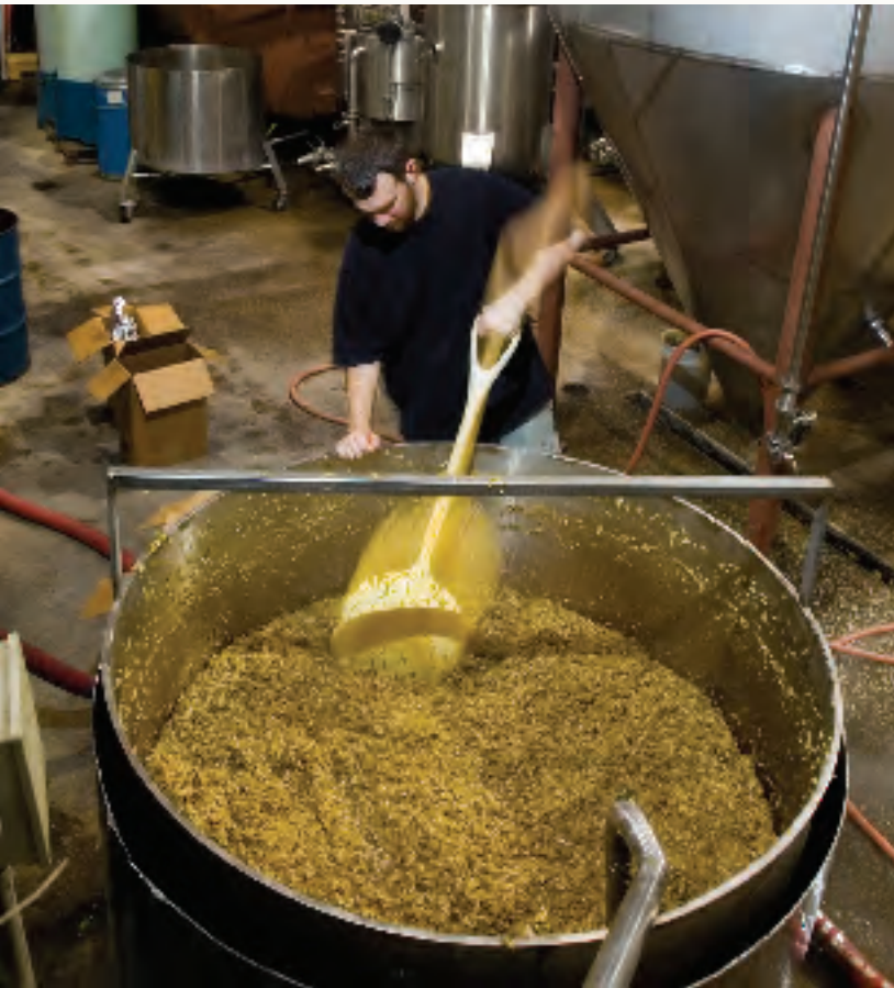
Above: Malt is ground to flour and mixed with water to produce mash, which is then sent to a lauter tun. Here large particles will settle off and a sugary liquid called wort is left. Right: After hops are added to wort, the mixture is sent to fermenting tanks for up to several weeks.
