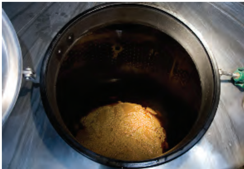
Partially germinated barley seeds are dried in a kiln to produce a finished malt. Temperature increases are gradual so that enzymes in the grain are not damaged. Higher drying temperatures produce deeper colored and more flavorful malts.
